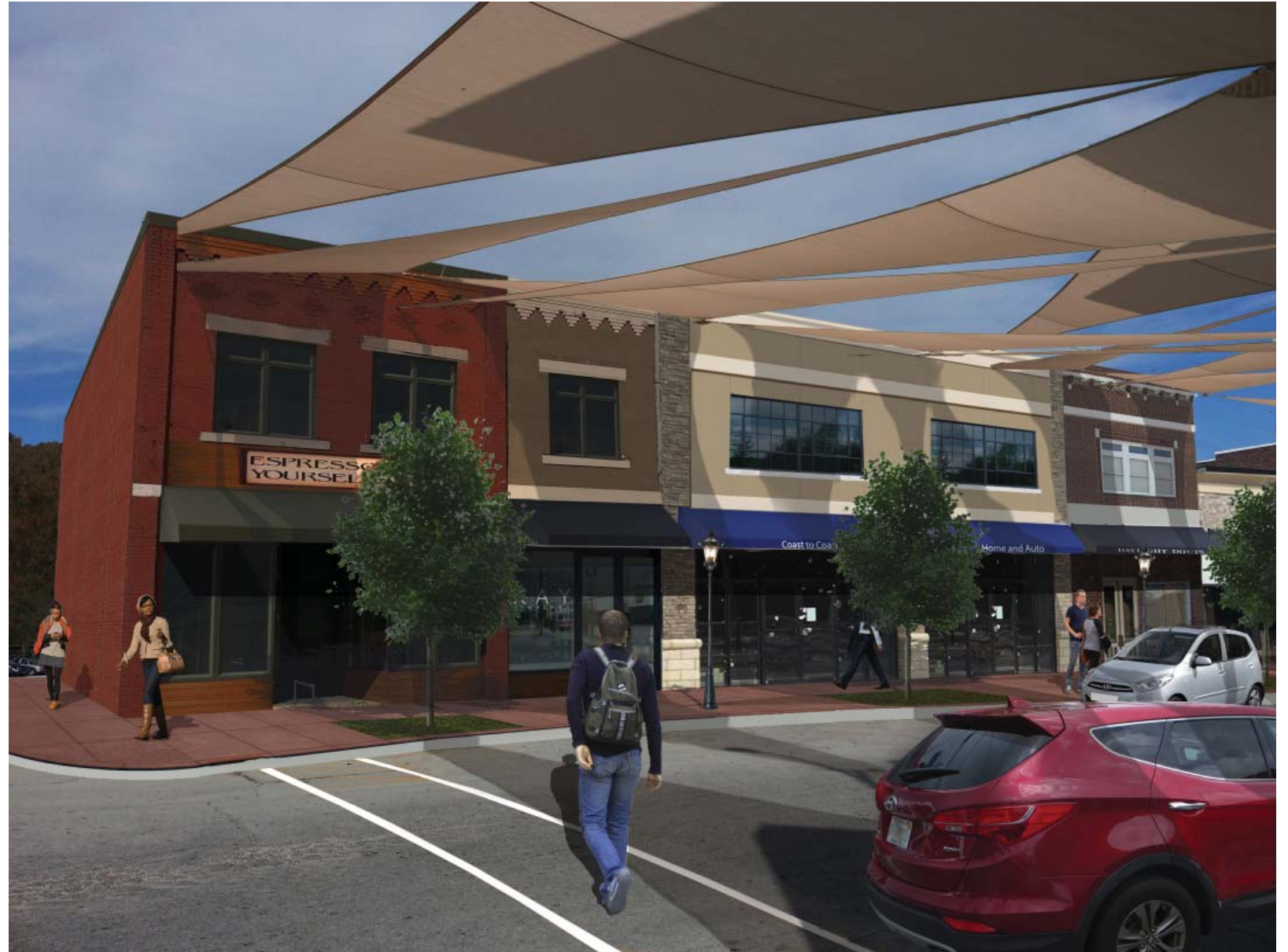
Main Street-West End (daytime) perspective depicting a rejuvenated facade with the introduction of tensile structures, awnings, pedestrian lighting, and trees.
